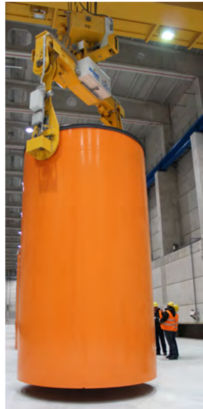
Panaudoto branduolinio kuro saugojimo konteineris CONSTOR RBMK1500/M2 Cask CONSTOR RBMK1500/M2 for spent nuclear fuel storage
